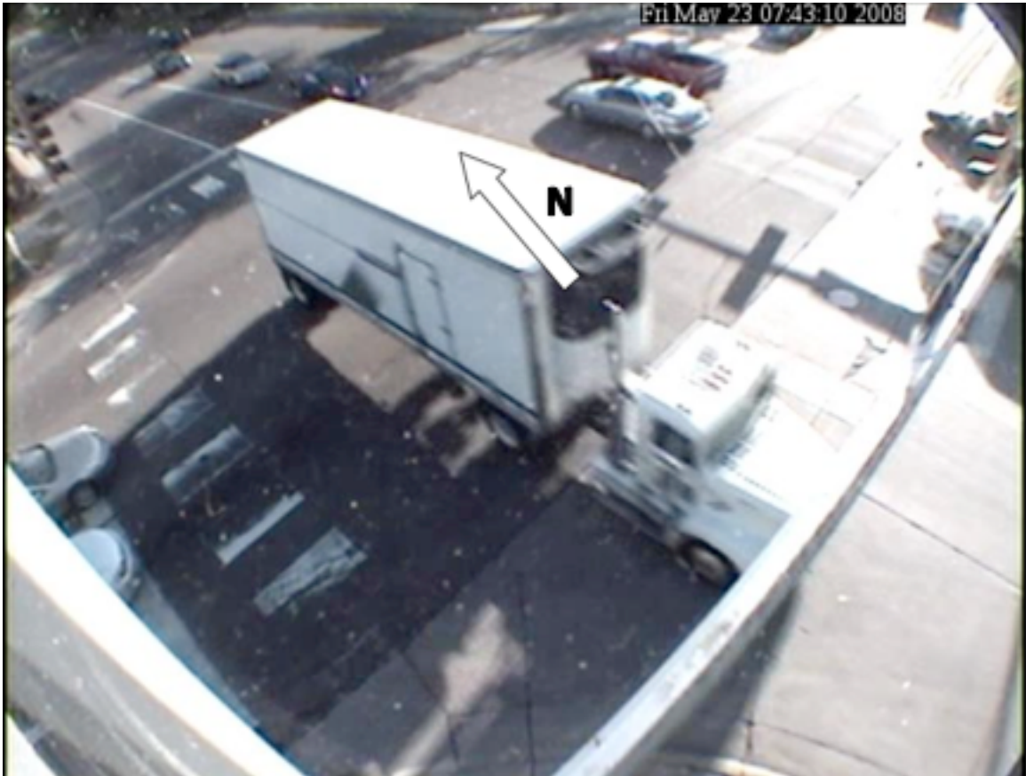
Figure 19: Site 2 - Occlusion analysis, trucks can create total occlusion.
