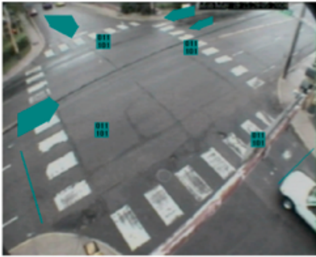
Figure 27: Site 1 – Configuration 5 – Combination of presence and directional detectors – one per lane with shadow processing.
