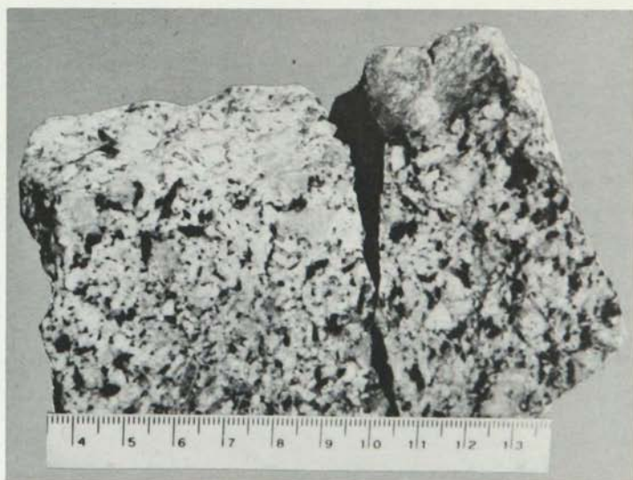
Figure 25. Textures characteristic of Farm Lake facies of Giants Range batholith. Note grain size, K-feldspar phenocrysts, slight foliation of hornblendes, euhedral feldspars and hornblende, lack of large quartz grains. M-7139 and M-7272, S. of Farm Lake.
