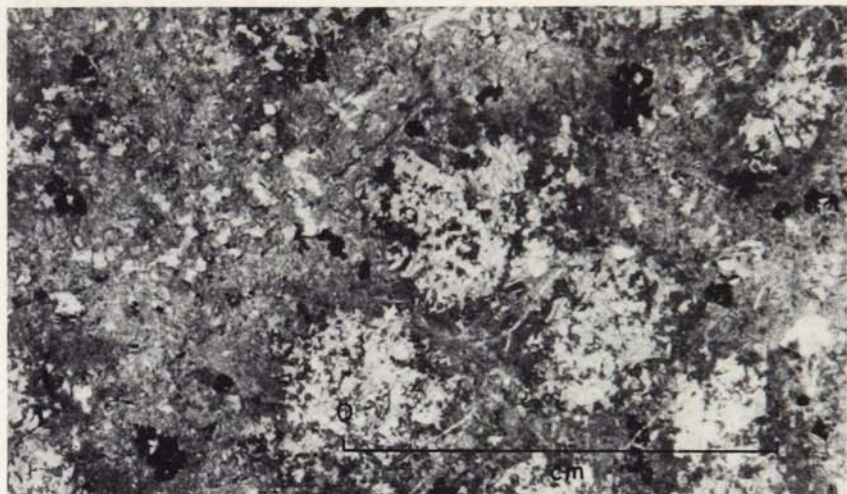
Figure 7. Photomicrograph of intrusive greenstone (analyzed) with relict ophitic augite oikocrysts, M-7286, sec. 9, 63 N/11 W.
