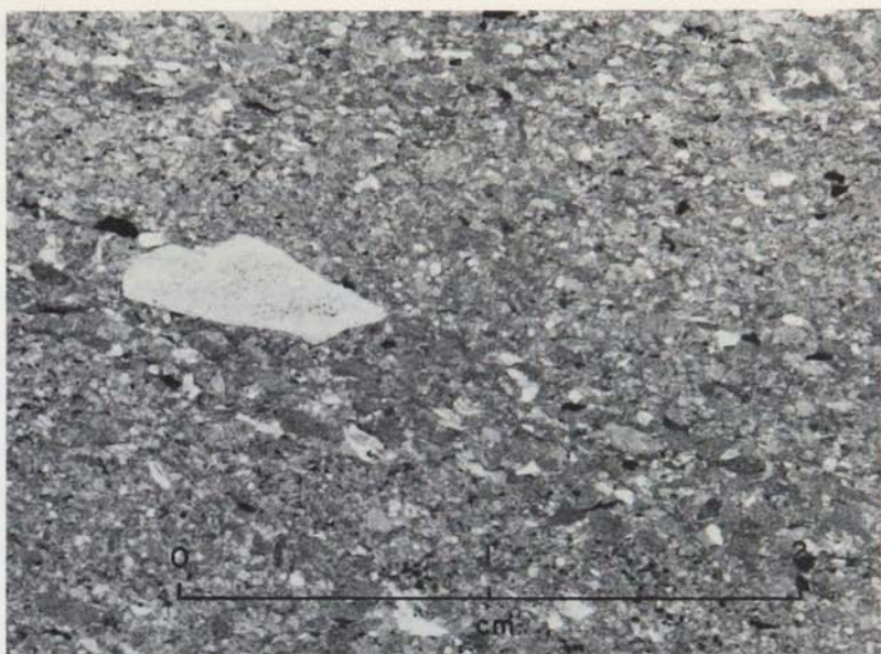
Figure 12. Photomicrograph of angular, gritty graywacke of Knife Lake Group. Note large chert clast and rare quartz; other clasts include greenstones, hornblende, plagioclase, and rare granophyre. M-7101, sec. 31, 64 N/9 W.
