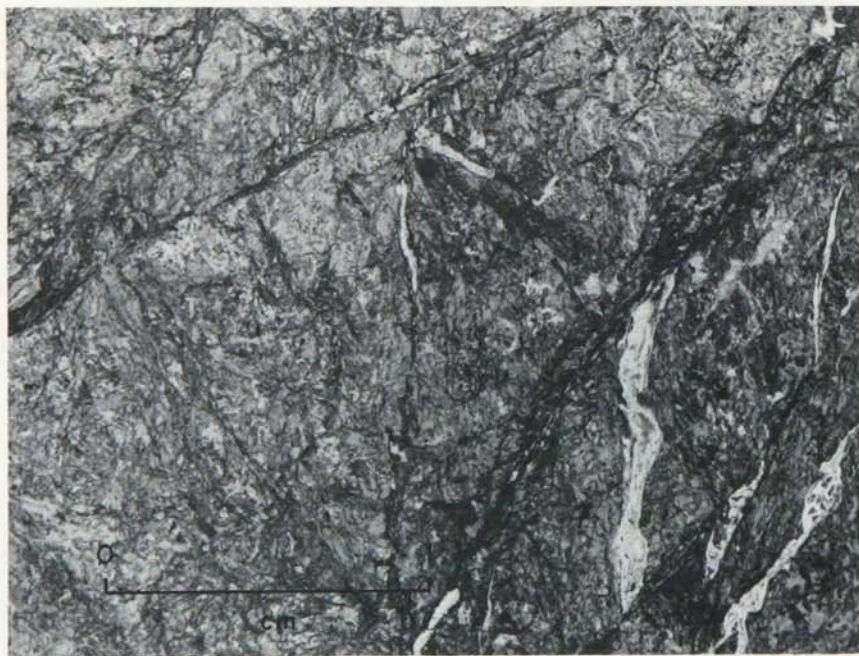
Figure 34. Photomicrograph of crushed, irregularly fractured metadiabase of Ely Greenstone at North Kawishiwi Fault, M-7593, sec. 28, 63 N/10 W.
