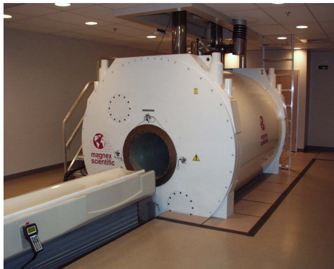
Figure 2.4: Photograph of the 9.4 T human scanner on which all experiments were run.
