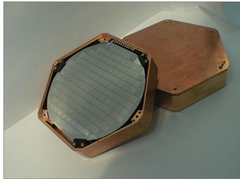
Figure 2.1: A ZIP detector with its hexagonal copper housing and photolithographic phonon sensors.
