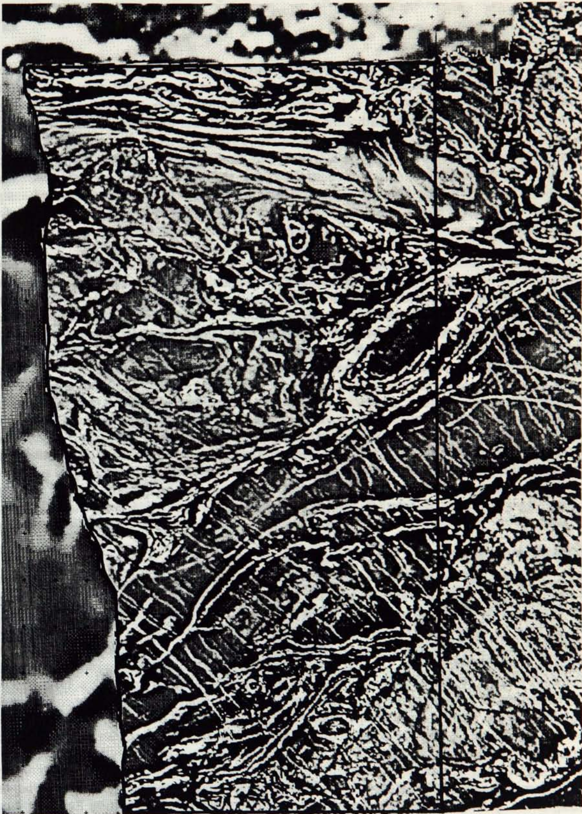
Figure 3. First vertical derivative map of reduced-to-pole magnetic anomaly data, northwestern Minnesota. The multitude of narrow, northwest-trending anomalies are produced by Proterozoic diabasic dikes that are not delineated on Figure 2. Scale is approximately the same as that of Figure 2 (1:1,131,000). Image produced by Val W. Chandler, Minnesota Geological Survey.
