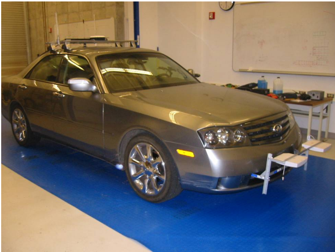
Figure 3.3: Test vehicle RFID reader antenna installation.
