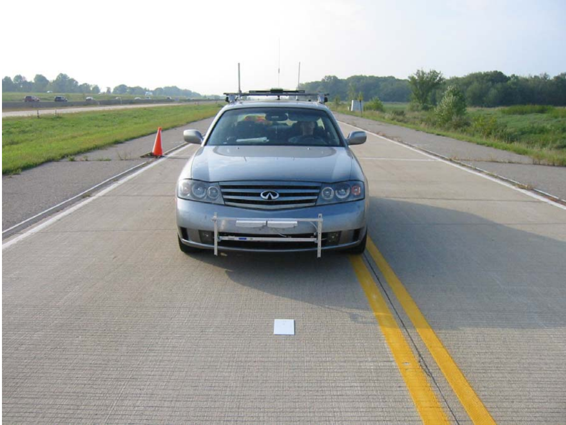
Figure 4.3: Picture showing RFID transmit antenna centered directly over RFID tag.
