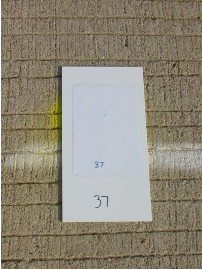
Figure 4.2: RFID tag bonded to Plexiglas.
