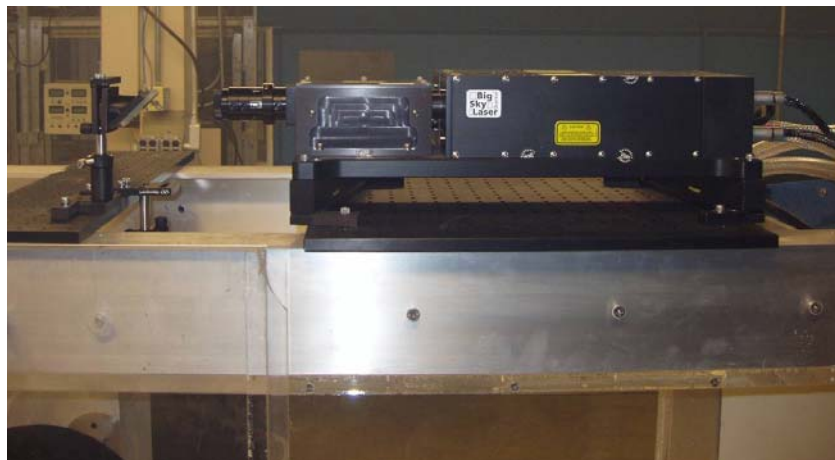
Figure 2.21: Laser used for high resolution PIV mounted to the top of the wind tunnel with light sheet optics and mirror.
