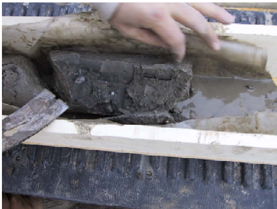
Figure 11. Rotasonic Drilling. A. Rig. B. Core Boxes. C. 4-inch Core
