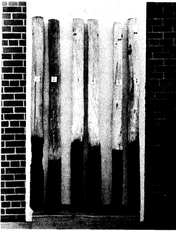
Figure 4. Appearance of some treated posts after 30 years in the Cloquet test plot. Posts #1 and #2 (left side) are jack pine; #3 and #4 are black ash; #5 and #6 are paper birch.
