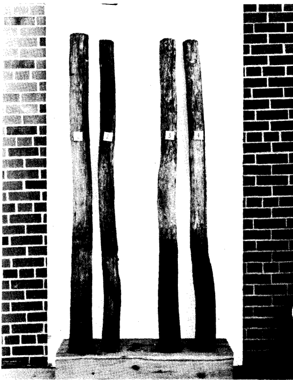
Figure 5. Appearance of some of the posts from the Waseca test plot after 25 years of service. Posts #1 and #2 (left side) are jack pine, #3 and #4 are black ash.
