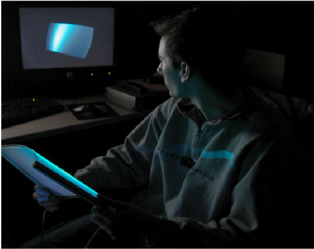
Figure 5.9: Another view of the flexible screen. The image displayed on the monitor is warped to display properly on the flexible screen.
