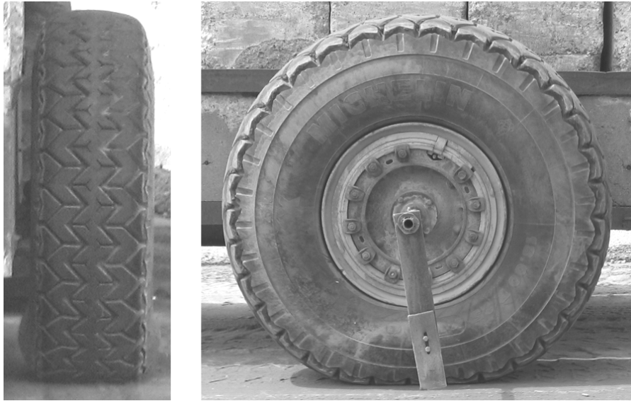
Figure 3.36. Photos of pneumatic tire for current test roller configuration
