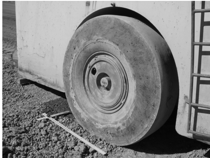
Figure 5.11. Test roller tire for test roller used at field sites
