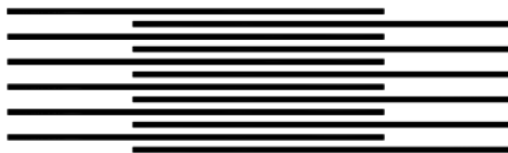
Figure III-8. 500 \mu\text{m} shadow mask. The electrode pattern used for the experiments of chapter V, VI, VII.
