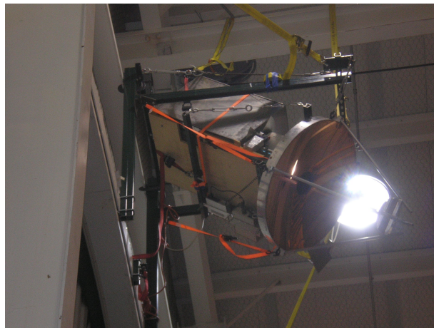
Figure 4.23: Integrated relative spectral response experiment with Ebert-Fastie monochromator mounted on the artificial planet (EFM on AP). Upper left – Conceptual design. Upper right – Code V simulation at 150 GHz. Right – EFM on AP as implemented in Ft Sumner.
