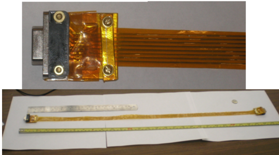
Figure A.5: Final configuration prior to installation in EBEX cryostat. End connectors are soldered to the small bit of copper sheathing exposed at each end of wires.
