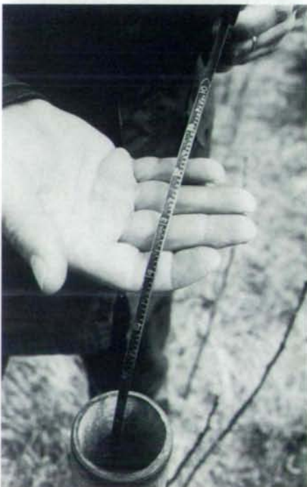
Measuring a water level in a monitor well.
