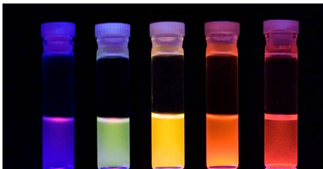
Figure 3.21: A photo of the red (675 nm), yellow (592 nm), green (572 nm) and blue (441 nm) light emissions from Si-NPs under the illumination of an UV lamp (excitation wavelength 365 nm). A 385 nm short-pass filter was placed between the UV lamp and each sample to remove any stray non UV light.
