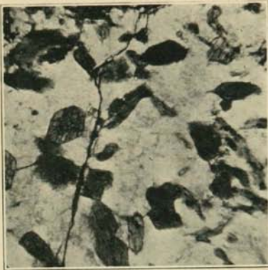
A. Shonkinite (Basswood type) near High Lake. The hornblende is poikilitically scattered in coarse feldspar.
