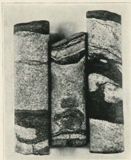
A. DRILL CORES OF IRREGULARLY BANDED TACONITE. BANDS CONSIST OF MAG- NETITE AND CARBONATE. THREE- FOURTHS NATURAL SIZE
