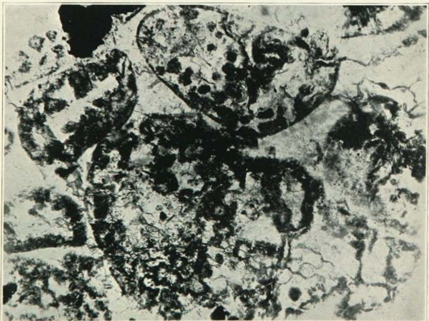
B. STRUCTURES SIMILAR TO A. CHERT RINGS SURROUNDED BY "DUSTY" BLACK RINGS. NUCLEI OF SAME MATERIAL. SOME ROUND DUSTY BLACK AREAS WITHOUT RINGS. COMPARE WITH PLATE XI, B. x 88
