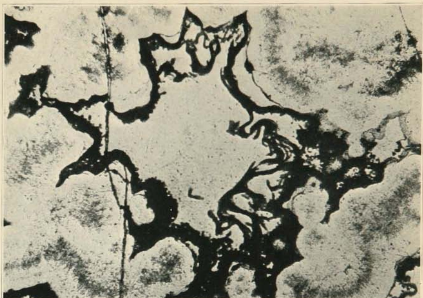
A. MICRO-ORGANIC STRUCTURES (ALGAE?) IN CHERT PEBBLES. THE CHERT SHOWS LARGE COLLOFORM OUTLINES. THE BROWNISH GREEN ORGANISMS (BLACK IN PICTURE) OCCUR ALONG THE OUTSIDE OF THE "SCALLOPS" IN A MATRIX OF THE SAME KIND OF CHERT. ORDINARY LIGHT. X 88. SLIDE M 904 a
