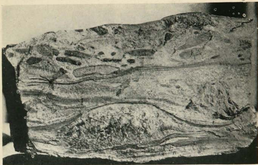
A. CHERTY TACONITE SPECIMEN SHOWING THE IRREGULAR BEDDING AND THE PARALLELISM OF THE FLAT PEBBLES OF THE CONGLOMERATE
