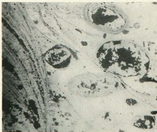
C. THIN SECTION, x 40. NOTE THE ZONES OF DEPOSITION EXTEND AMONG AND IN SOME CASES AROUND THE PEBBLES. THE IRON OXIDE IS IN LAYERS ALTERNATING WITH SILICA AND SEEMS CLEARLY A PRIMARY PRECIPITATE
