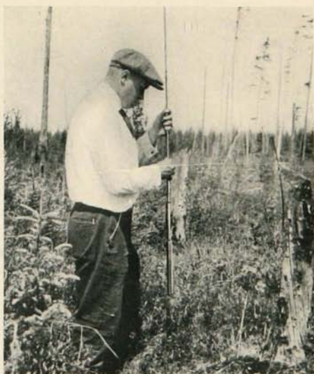
B. DRAWING UP THE PEAT SAMPLE WITH THE DAVIS PEAT SAMPLER. THE SAMPLER HAS JUST BEEN PULLED OUT OF THE HOLE WITH THE CYLINDER FULL OF PEAT
