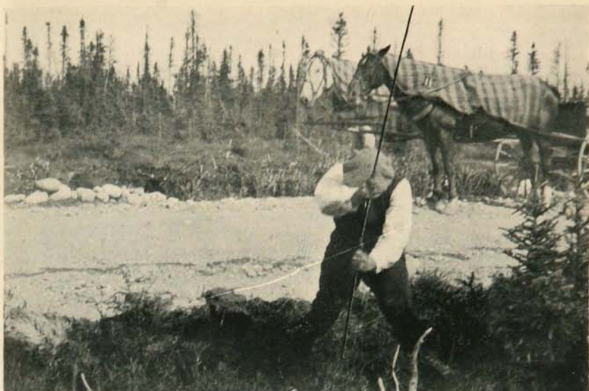
A. PUTTING DOWN TEST HOLES IN A PEAT BOG WITH THE DAVIS PEAT SAMPLER. THIS SHOWS THE OPERATION OF FORCING THE RODS DOWN THROUGH THE PEAT
