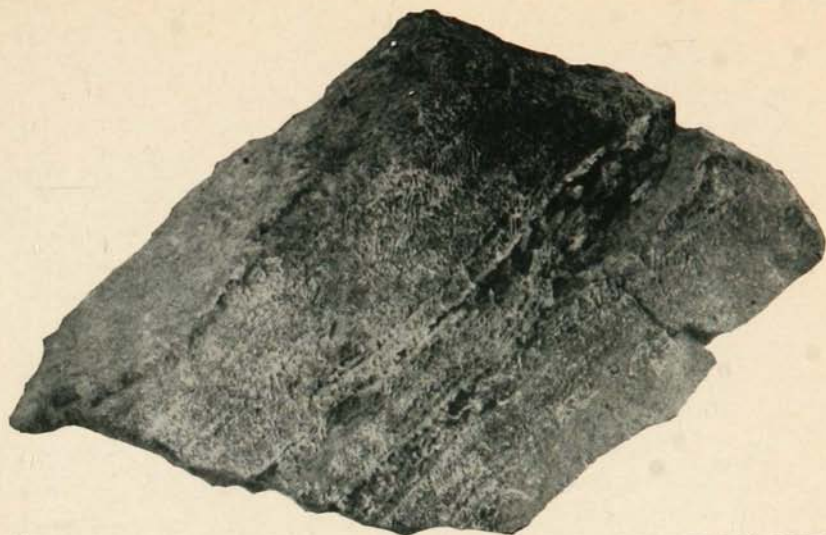
A. WASH ORE SHOWING POROSITY DUE TO DISINTEGRATION AND REMOVAL OF CHERT AFTER APPLEBY AND NEWTON
