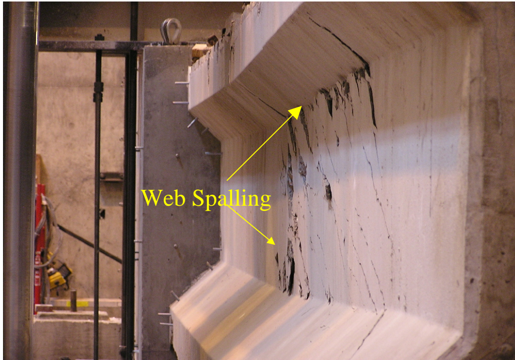
Figure 6.33 Web Crushing (Specimen II)
