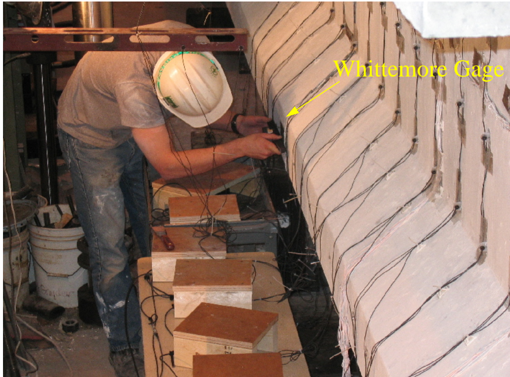
Figure 4.20 Measurement of DEMEC Points
