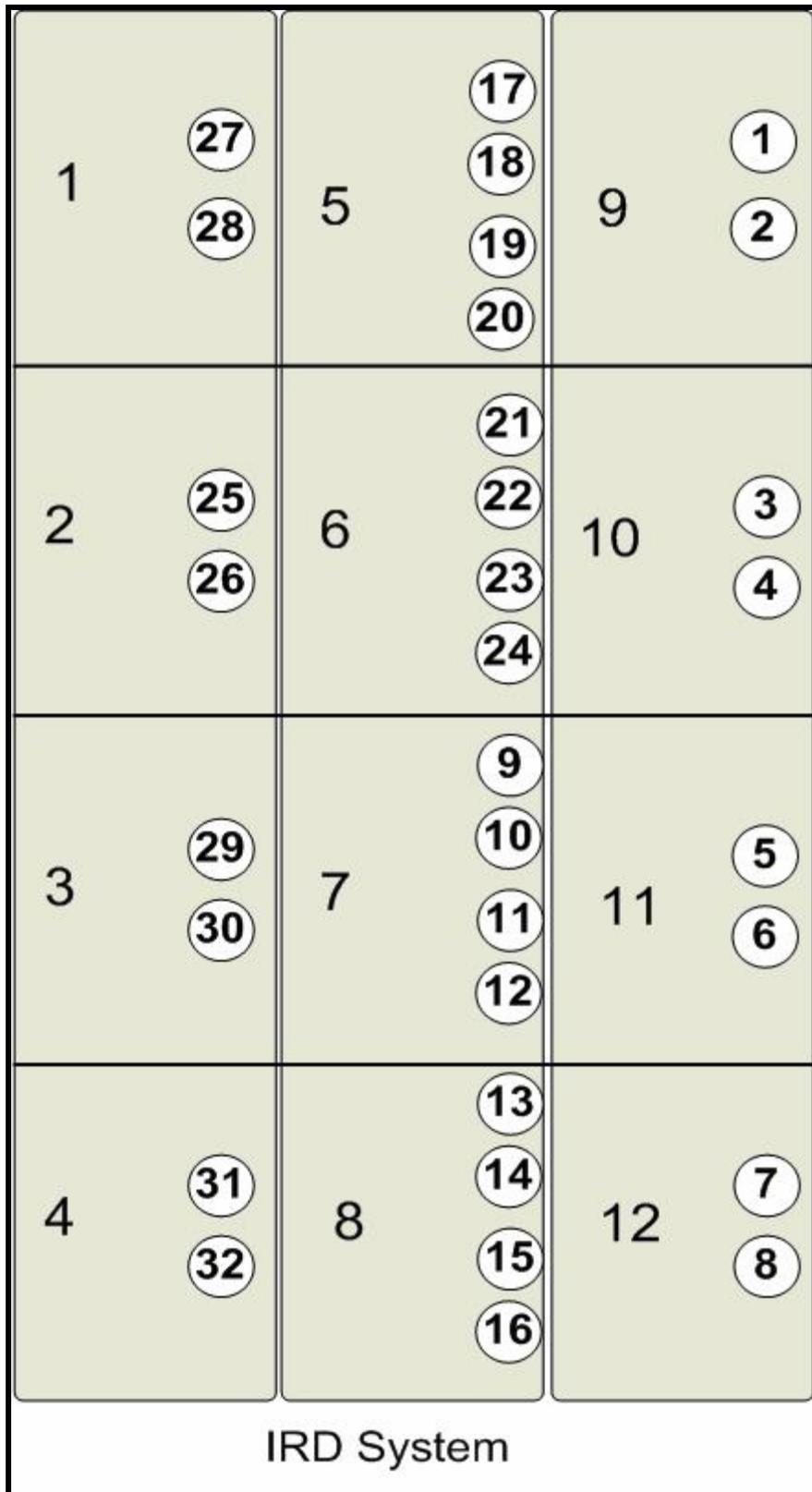
Figure 34: IRD panel and cable numbering scheme
