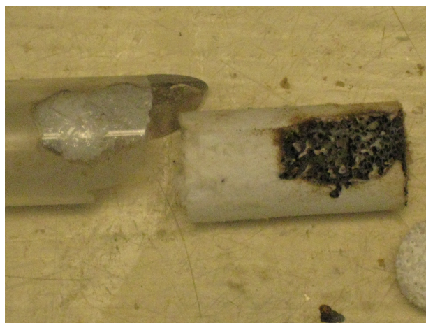
Figure C.7: Photo depicting a catalyst bed near its used reactor. The reactor, used for the CPO of 50 wt% pine pyrolysis oil, 50 wt% methanol, began leaking before breaking on disassembly. The catalyst is exposed where there should be FiberFrax ceramic paper; a similar shape is burned into the quartz reactor. The ceramic paper exothermically melted onto the catalyst, producing glassy bulbs appearing on the side of the exposed bed.
