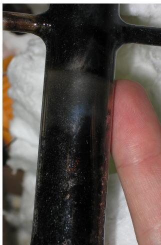
Figure C.2: Photo of a coked reactor after the CPO of 50-50 wt% poplar pyrolysis oil and methanol, which ran autothermally for a short while before shutting down due to coke formation. A finger is resting on the position where the catalyst bed is, and the difference in color may indicate that the catalyst is not as coked as the rest of the reactor.
