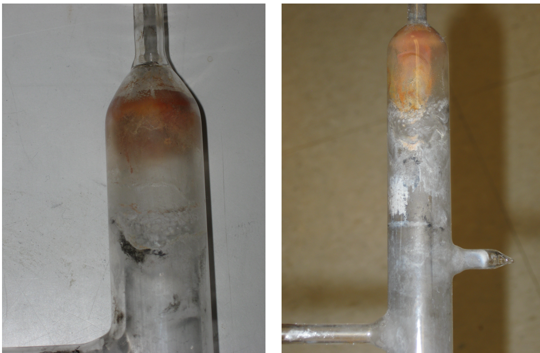
Figure 5.9: Red ash was deposited upstream of the reactors for both the 375 hr (left) and 450 hr (right) experiments. Etching is also apparent in the quartz swirls below the ash deposit for both reactors.
