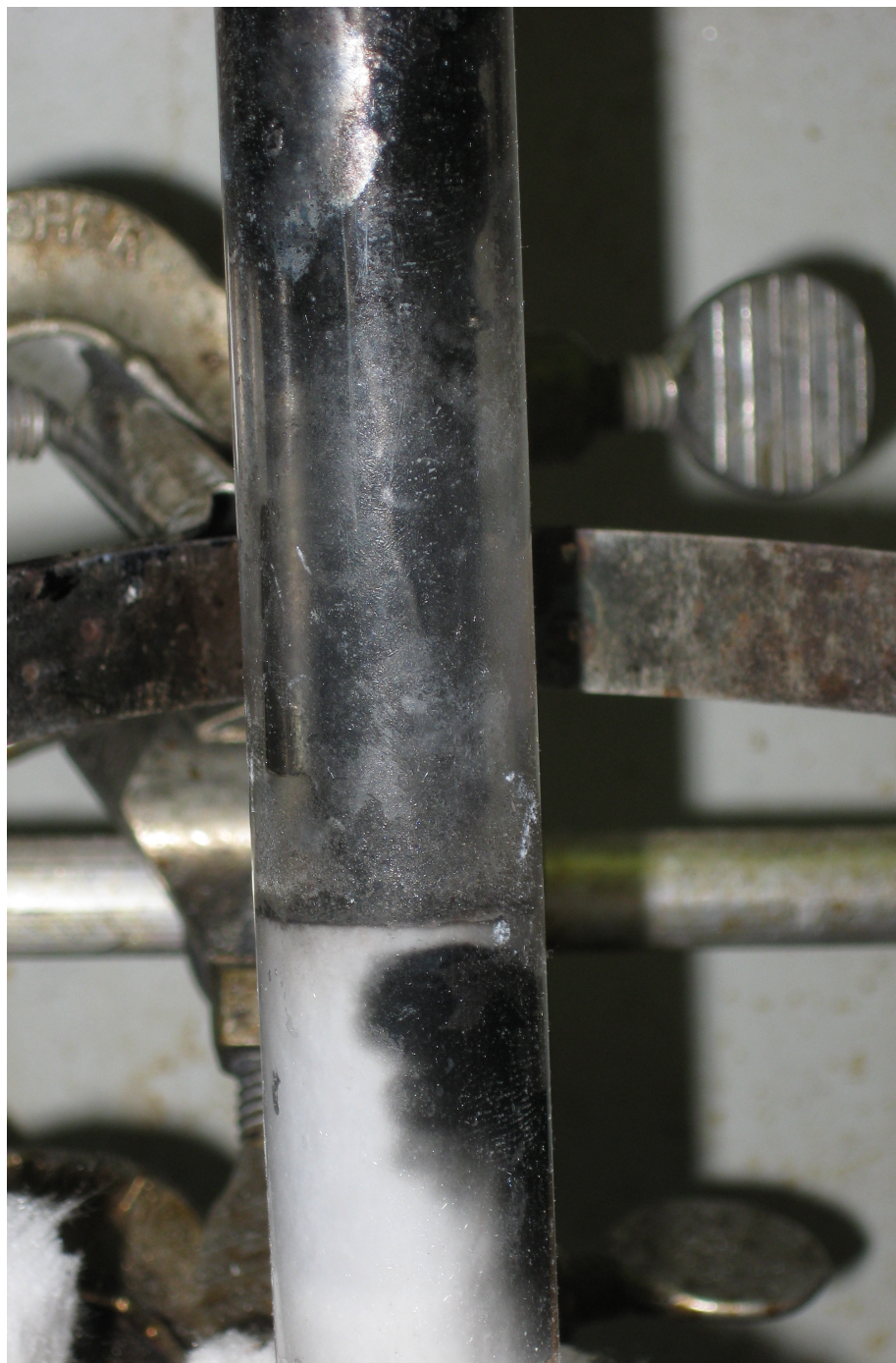
Figure C.4: Photo depicting the lack of carbon deposition near the inlets and catalyst. This reactor was used in the partial oxidation of pure pine pyrolysis oil assisted by a furnace. Coke is apparent far upstream of the catalyst at the top of the image, deposited by recirculation of pyrolysis oil aerosol. However, near the catalyst a 1/8" tube can clearly be distinguished, as can the 5/16" jacket of the water-cooled nebulizer.
