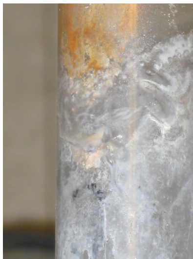
Figure C.8: Close-up of the quartz etching in the reactor from the 450 hour time on stream test of the RFV of glycerol. Red ash deposit is visible above the smoky bubbling of the reactor.
