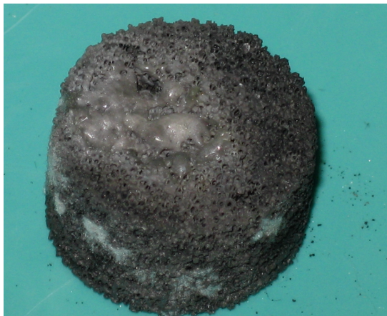
Figure C.6: Rh-Ce catalyst used in the CPO of 50 wt% poplar pyrolysis oil with methanol shows the deposition of a glass due to introduced impurities.
