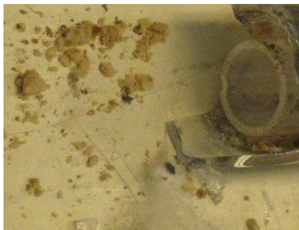
Figure C.5: Ash accumulation from pyrolysis oil is apparent in this reactor. The pyrex annulus is used to insulate the jacketed nebulizer from the hot furnace, shown here from the CPO of 50 wt% pine pyrolysis oil, 50 wt% methanol. All of this ash is upstream of the catalyst, suggesting that this type of ash accumulation can be eliminated with reactor design.
