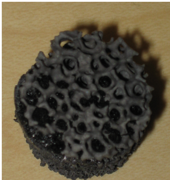
Figure C.3: Photo depicting a 20 ppi catalyst used for the CPO and reforming of pyrolysis oil. This catalyst was at the front of the bed and its pore size was too large for the noble metal to react this coke, which visibly accumulated in the pores. Water was added in this experiment in the amount S/C = 3.0 , resulting in cooler temperatures that can promote coke deposition.
