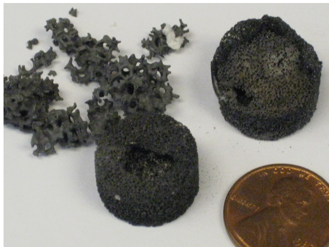
Figure C.1: Photo of monoliths which have lost mechanical stability. In this image, a 20 ppi catalyst has crumbled after use in the CPO of bio oils. Two 80 ppi catalysts are also shown with holes punched into the monoliths after CPO of bio oils. It has been observed previously that the CPO of oxygenated functional groups can result in catalyst disintegration (Chapter 4, [159, 64, 47]). The cause is as yet unknown, but is thought to be due to silica leaching from the support. Incidentally, the top right monolith also shows coke deposition - the black fringe at top - and slagging, the white patch near at the 2 o'clock position.
