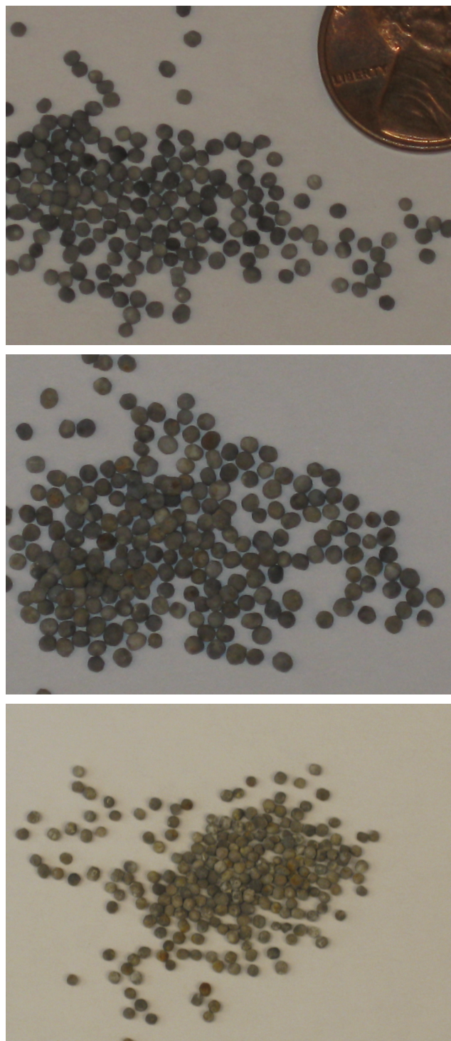
Figure 5.10: Catalyst for the CPO of glycerol. The top image shows unused catalysts: all are grey. The middle image shows catalysts used in the 375 hour RFV of glycerol experiment, and the bottom image depicts catalysts used for 450 hours. Red and brown deposits are visible on the used catalysts, the color matching that of the deposit on the walls of the reactor.
