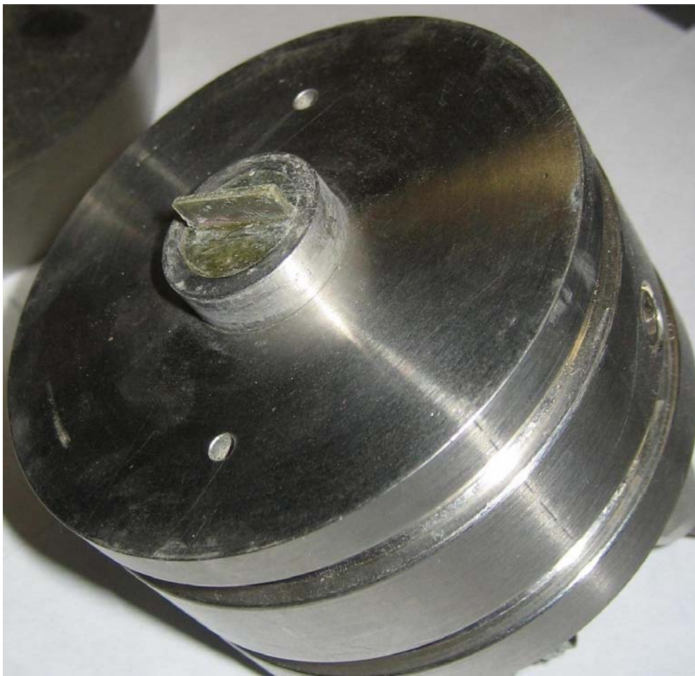
Figure 2.1. Bender elements housed in resilient modulus platens.
