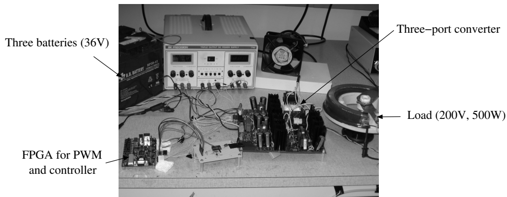
Figure 4.17: Hardware setup for testing the series resonant three-port converter
