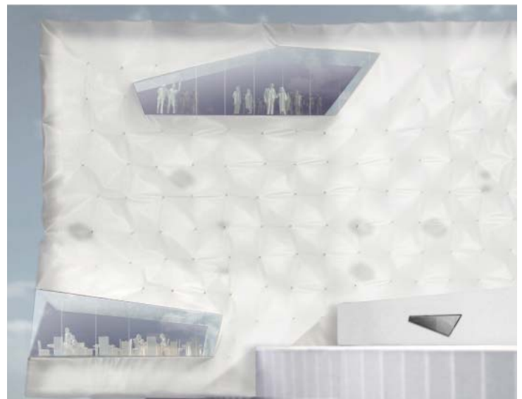
7.5. Right. A vellum model explores the transparency in the cladding. This iteration would have allowed light to pass through the building in limited amounts revealing the floor plates and massive structure of the building.
