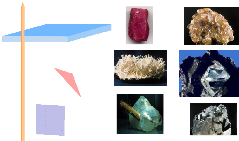
Figure 1-5. (Left) Idealized examples of some of the many habits observed in crystals, including needles (formally: “acicular”), plates (formally: “tabular” or “lamellar”), cubes, and octahedra. (Middle and Right) Photographs of minerals exhibiting various natural habits. All photographs used in this figure are public domain. Source: http://en.wikipedia.org/wiki/Crystal_habit Last accessed: 2 April, 2009.
