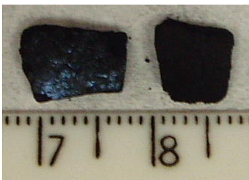
Figure 3.4. Photograph of 3DOM tungsten monoliths produced from a 2 M APTA1 precursor solution. The sample produces an opalescent blue color on the top surface.
