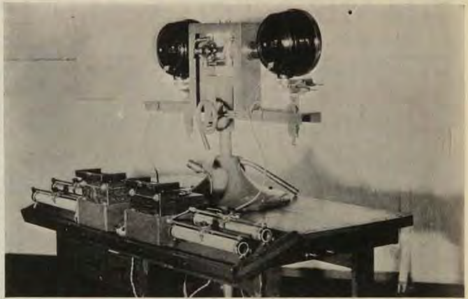
A close look at the headlamp stand with lamps to be tested, shows us that the lamps may be placed in any position required for adjustment. In order to obtain the precision motions necessary each lamp is mounted on jeweler's lathe beds. Note the recording instruments.
