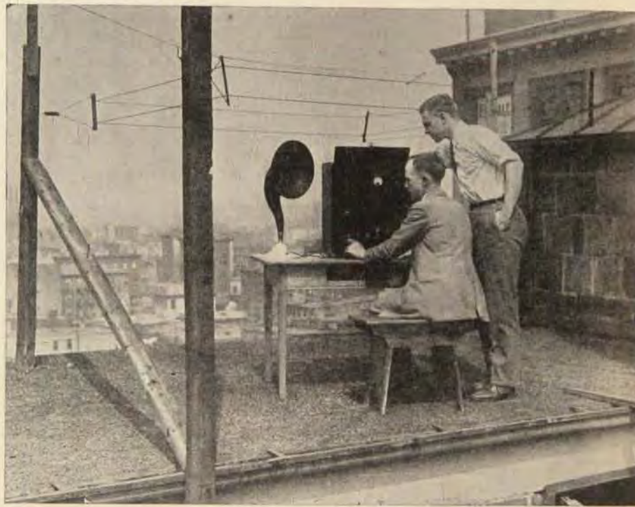
Just what horizontal waves will do over long areas has not been determined according to David Grimes. Here Grimes (standing) is seen with one of his associates experimenting with a horizontal radio receiver on the roof of his New York laboratory. Note particularly the double-strand type of aerial and method of insulation.
