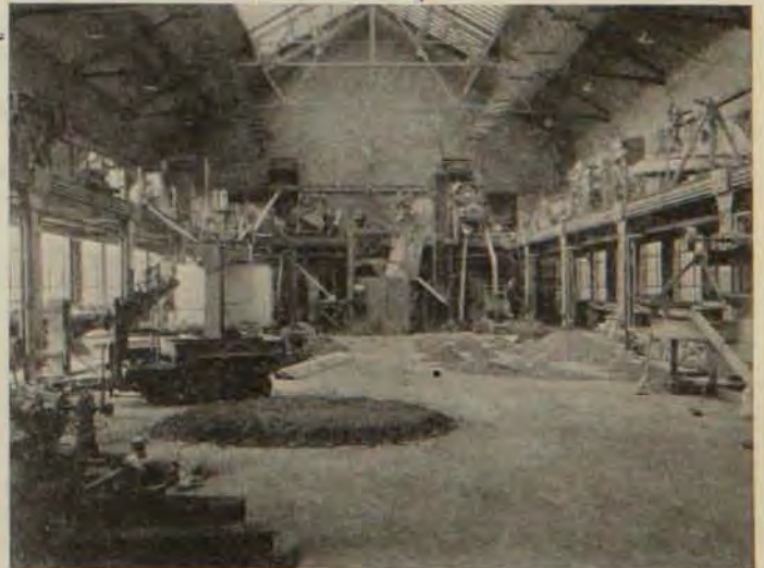
Here we see the machinery on the floor and in use. Ore comes through the two openings in the further wall from storage bins and is fed to the various machines for further treatment.
