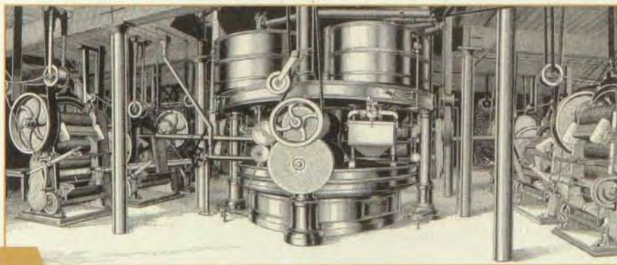
One of the chocolate machines at the Walter Baker & Company manufactory in Dorchester, Massachusetts, circa 1890. The machine could produce 10,000 pounds of chocolate daily.
