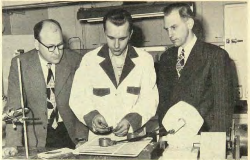
In the Institute of Technology work-study program Hartley Conrad, center, mechanical engineering student on the Minneapolis campus, works part time at the Coolerator Co. of Duluth for experience training. With John A. Forsman, Coolerator chief chemist, left, and Dr. Clarence B. Lindquist, UMD engineering department head, watching, Conrad takes a micrometer abrasion reading to determine wear on an electric refrigerator.
