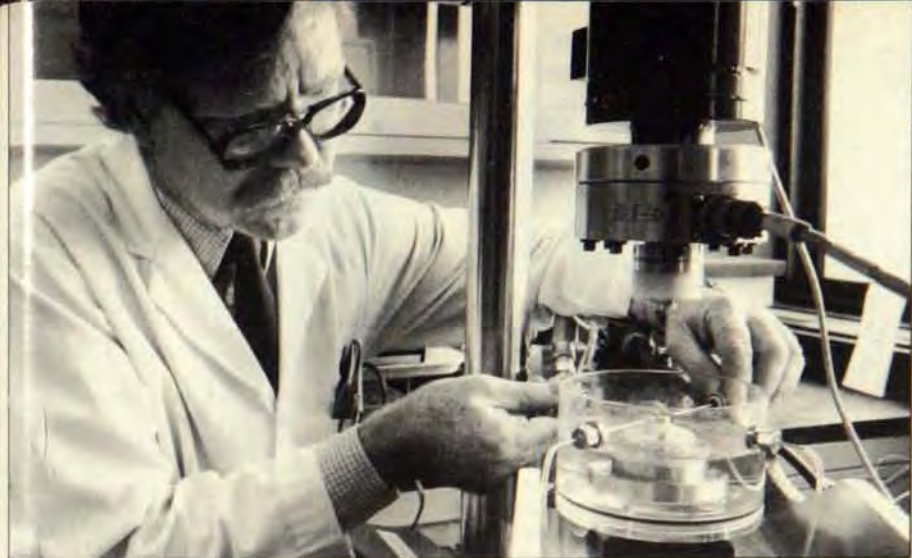
Ralph DeLong adjusts ART, an artificial chewing machine used to test new materials for dental work.
