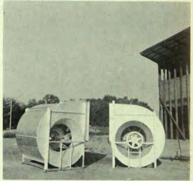
TWO HUGE fans in the building will help to make a complete exchange of air every six minutes in the winter months.
