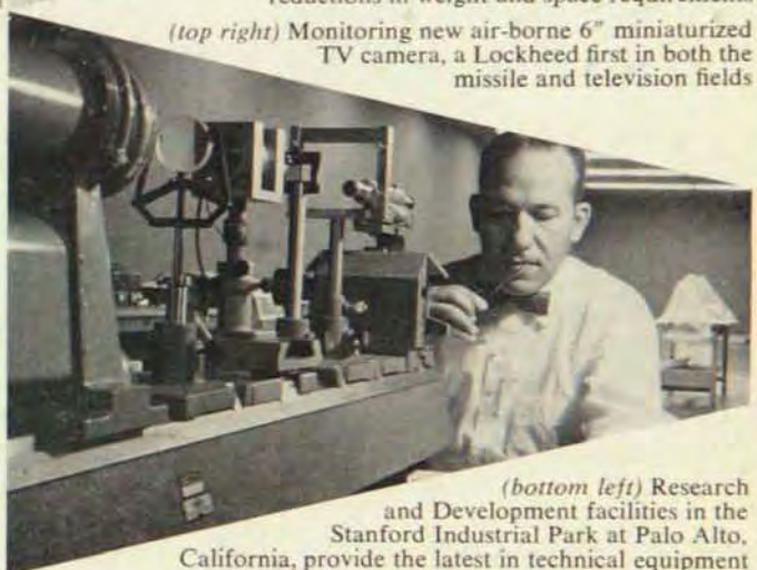
(bottom right) Setting up a diffraction image for a research study in infrared optics
