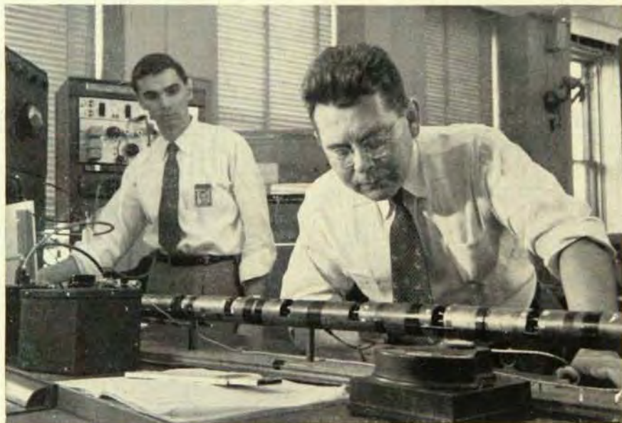
RELAYS VOICES UNDER THE SEAS. This is one of the repeater units in the new underseas telephone cables. These voice boosters make it possible for you to telephone Great Britain and Hawaii as clearly as you call across town. Developed by Bell Telephone Laboratories after many years of research. Made to entirely new precision limits by Western Electric.
