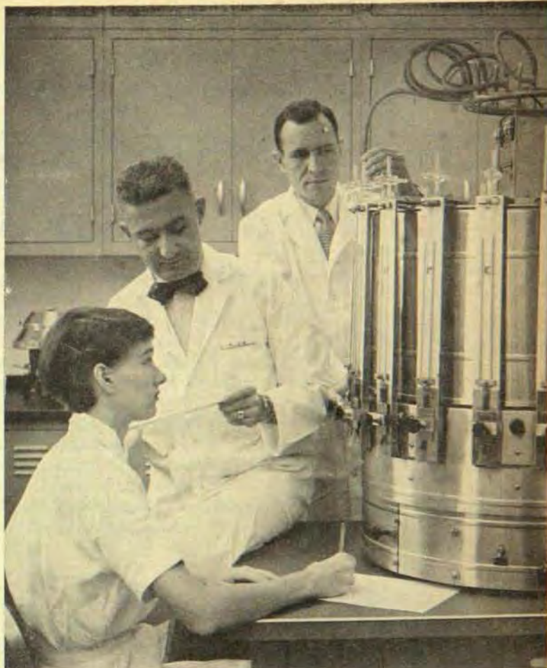
Equipment, such as this Warburg respirometer used to study metabolism of bacterial cells and how they produce and absorb gases, makes the Memorial bacteriology laboratory a model of its kind.
