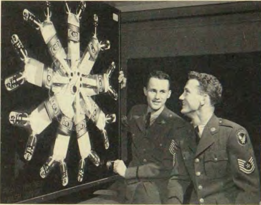
"It's all very simple," says Cadet Master Sgt. Bill Pearce of the University Air ROTC, left, as he uses a mockup to explain the operation of an aircraft radial engine to Cadet Technical Sgt. Tom Mulcahy. Tom's expression indicates he doubts the simplicity part. The engine is of the type used in T-6 trainer planes. Pearce is from Faribault, Minn. Mulcahy lives in Minneapolis.
