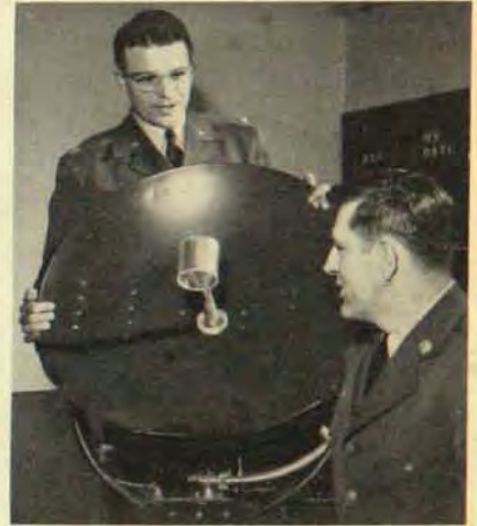
An airplane's far-sighted eye, its radar, is shown by Maj. Walter H. Grierson, U. S. Air Force, to Cadet Capt. Edward H. Johnson of Eau Claire, Wis. Mounted in the nose of the plane, the spool cylinder on the shaft is the receiving antenna. Outgoing impulses come through the dot-like spot on the front of the receiving antenna.
