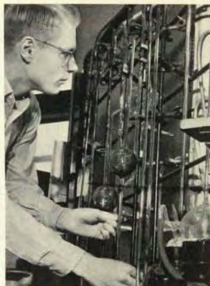
Royce Freese, chemical engineering student, studies the operation of a newly developed apparatus for gas absorption measurement of the product of crushing operations. The measurement procedure is useful in determining the efficiency of equipment used in ore treatment and similar fields.
