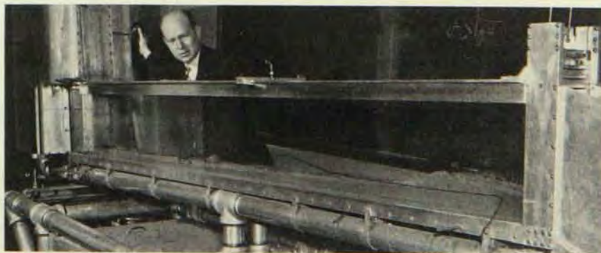
At the St. Anthony Falls Hydraulic Laboratory, Lorenz G. Straub, laboratory director, operates a demonstration flow channel used in hydraulic study.
