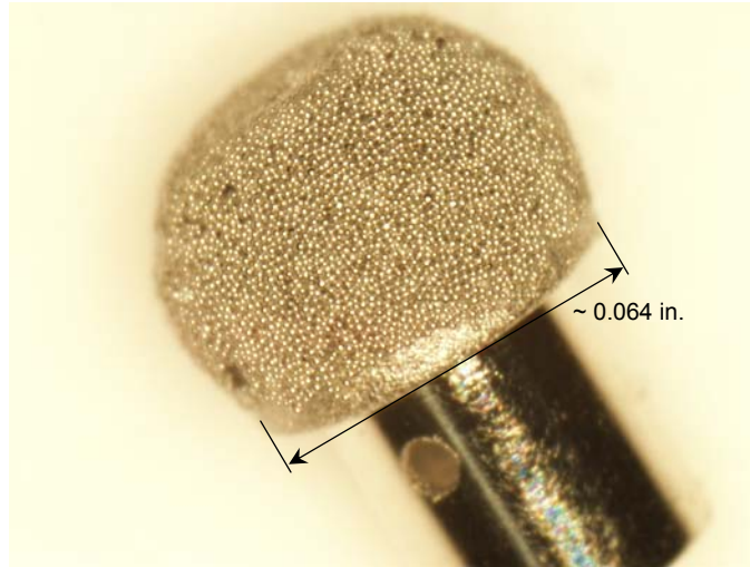
Figure 12: Image taken under light microscopy of an example electrode base successfully coated with platinum iridium microspheres after setting of the binder.
