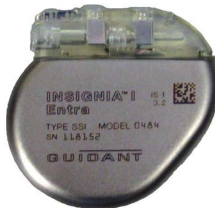
Figure 21: Image of INSIGNIA™ model pacemaker utilized for electrical data acquisition in the chronic animal study.
