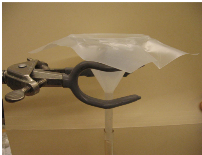
Figure C.7. Preparation of liquid enclosure for testing microcantilevers in liquid environments
