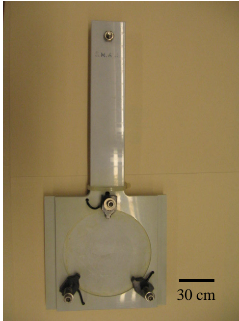
Figure B.2. Optical image of wafer holder (cathode) for electroplating
