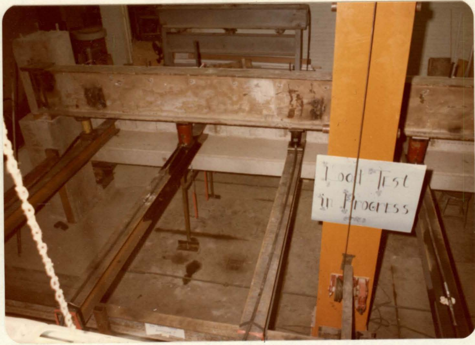
Photograph #1 - North-One-Half of Test Setup, Front-View, Displaying Simulated Double-Tee, Loading Beams.
