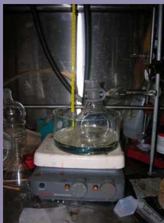
Set up for reactive monomer of 1,2:5,6-di-O-isopropylidene- \alpha -D-glucufuranose synthesis
