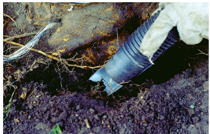
Fig. 30—A small trowel and vacuum may be used to loosen and remove soil during a nondestructive examination.
