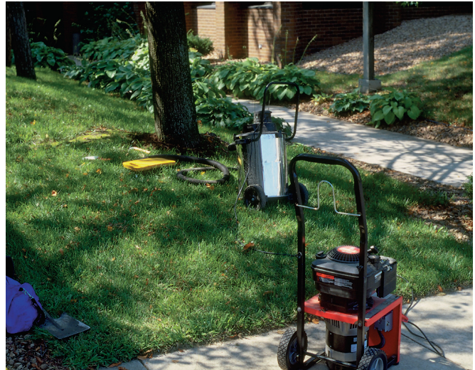
Fig. 27—Larger, more extensive and nondestructive examinations justify the use of wet/dry vacuums and portable generators. These tools greatly reduce the amount of time required to remove soil from the examination area.
