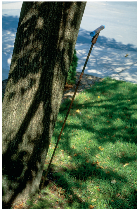
Fig. 28—Probing the soil area near the root flare can help determine the extent (depth and width) of the examination and if it's warranted.
