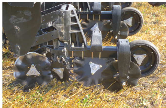
Photo 4. Coulters-only strip-till unit. Other designs are also on the market.
