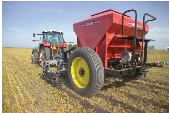
Photo 8. Applying banded P and K fertilizer with the strip-till pass.
