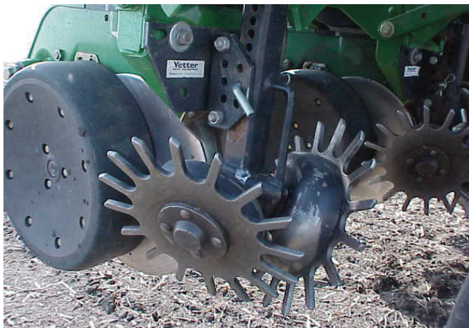
Photo 7. Residue managers on the planter to clear the row.
