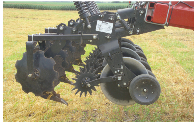
Photo 3. Typical strip-till unit with cutting coulters, residue managers, mole knife, and berm shapers.
