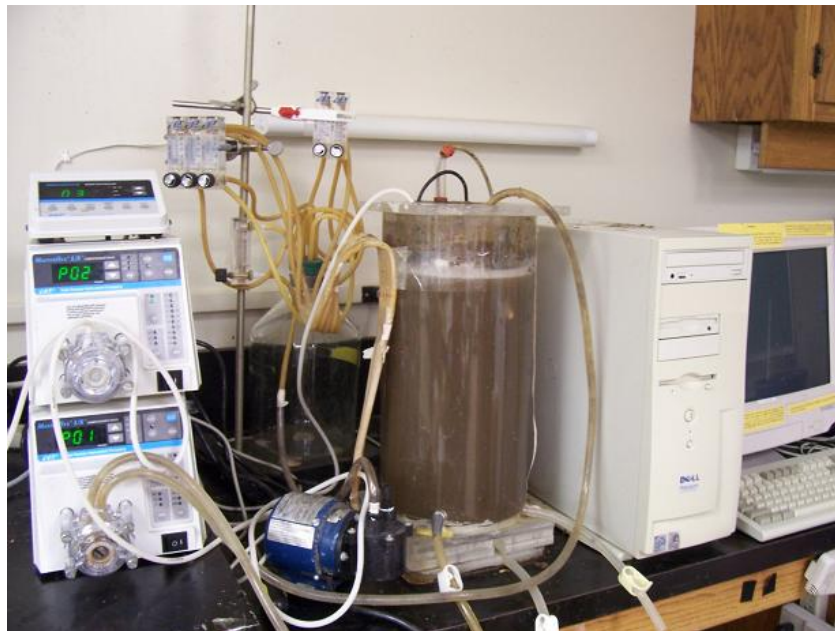
Fig. 2.2 The real system of the nitritation SBR (Omitting the influent and effluent tanks).
