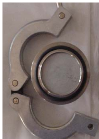
Figure 3.1. 5 micron stainless steel filter shown inside KF50 retainer ring with O-ring gasket (ring and gasket are sitting on a KF50 flange)
