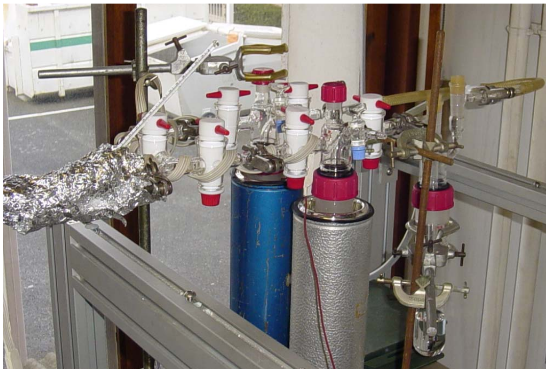
Figure 3.3. Trapping set-up showing bypass line (behind, dark dewar) and mass transfer trapping line (closer, light dewar and bubbler trap on right)
