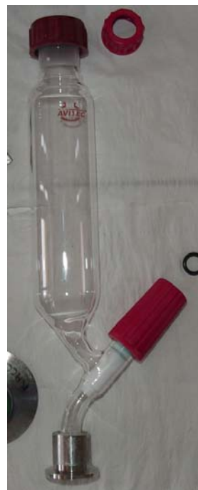
Figure 3.2. Precursor loading vessel for protecting reactive precursors from atmosphere (scale - bottom flange is KF25)
