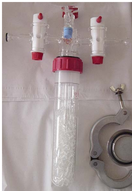
Figure 3.4. Dry, cold trap filled with small glass tubing pieces (scale – flange shown on right is KF50)
