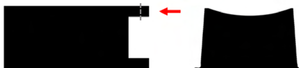
Figure 26: Sidewall angles and lips on electroplated nickel parts that result from the fabrication process. These fabrication artifacts are a function of the processing and vary both across a single wafer and between wafers fabricated at the same time. The effects are exacerbated by the thick film resist used to fabricate the photoresist molds, which are discussed in a later chapter.
