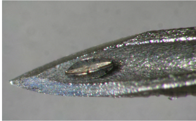
Figure 14: 500 \mu\text{m} long biomicrorobot in the tip of a 0.9 \text{ mm} needle (20 gauge).
