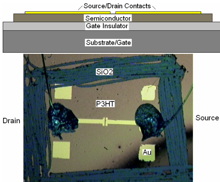
Figure 3.3: The P3HT FET structure and picture of actual device.
