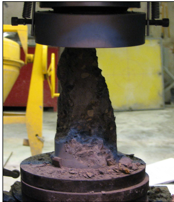
Figure D-2 Concrete compressive strength test
